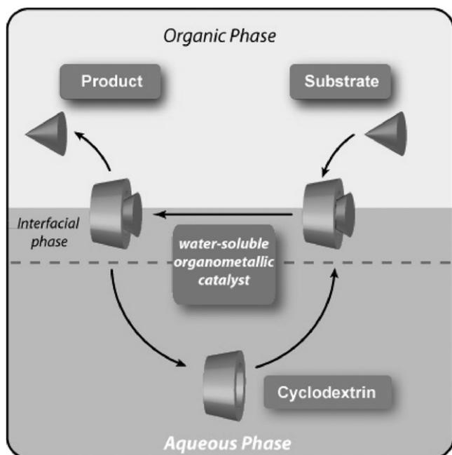
**Fig. 1.** Principle of interfacial catalysis in biphasic aqueous organometallic process promoted by CD.
