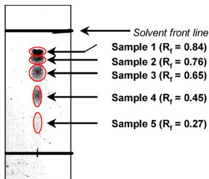
**Fig. 2.** Thin-layer chromatogram obtained from a commercially sample of RAME- $\beta$ -CD (mobile phase: CH<sub>2</sub>Cl<sub>2</sub>–MeOH, 8:2, v/v; stationary phase: silica plate; developed by heating the TLC plate after immersion in methanol–sulphuric acid, 9.5:0.5, v/v).
