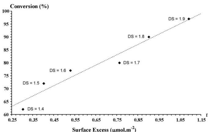
**Fig. 3.** Conversion in hydroformylation of 1-decene as a function of surface excess ( $\Gamma$ ) [conversion (%) =  $39.984 \times \Gamma$  ( $\mu\text{mol}\cdot\text{m}^{-2}$ ) + 53.038;  $R^2 = 0.9499$ ].
